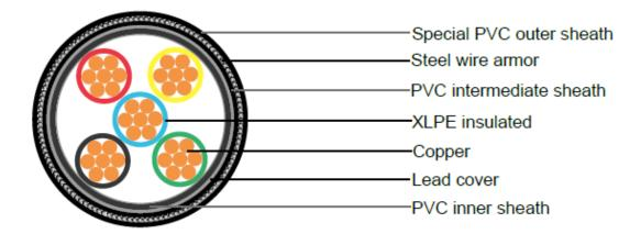
**Conductor:** Plain copper wire conductors to IEC 228, class 2 (stranded).
